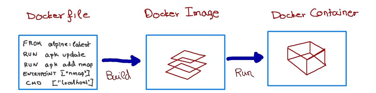
Docker Image is a template aka a blueprint to create a running docker container. Docker uses the information available in the Image to create (run) a container.
