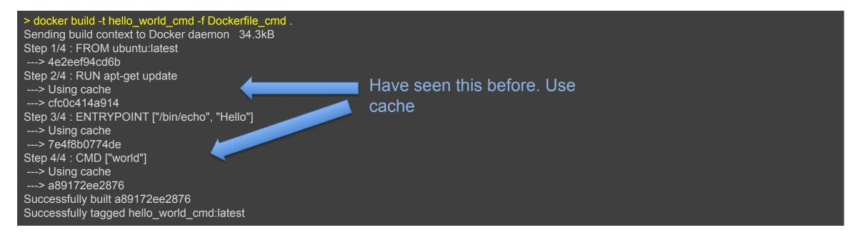
As you can see that the image was built using the existing layers from our previous docker image builds. If some of these layers are being used in other containers, they can just use the existing layer instead of recreating it from scratch.
