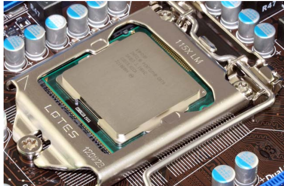
CPU mounted in a socket on the motherboard
