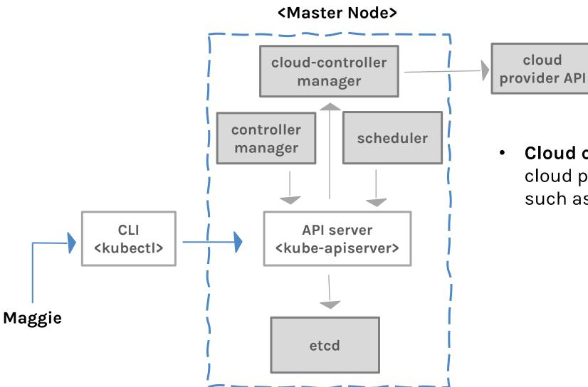
Cloud controller communicates with cloud provide regarding resources such as nodes and IP addresses
