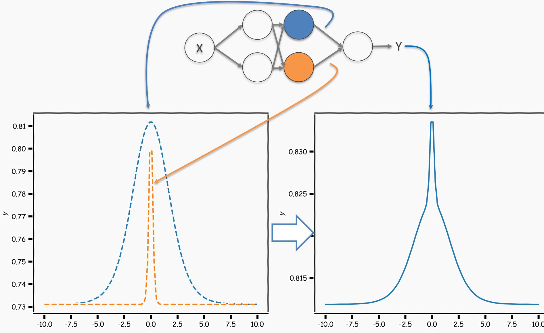
Adding layers allows us to model increasingly complex functions
